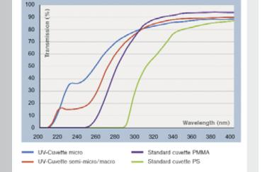
Transmission curves of different cuvettes
